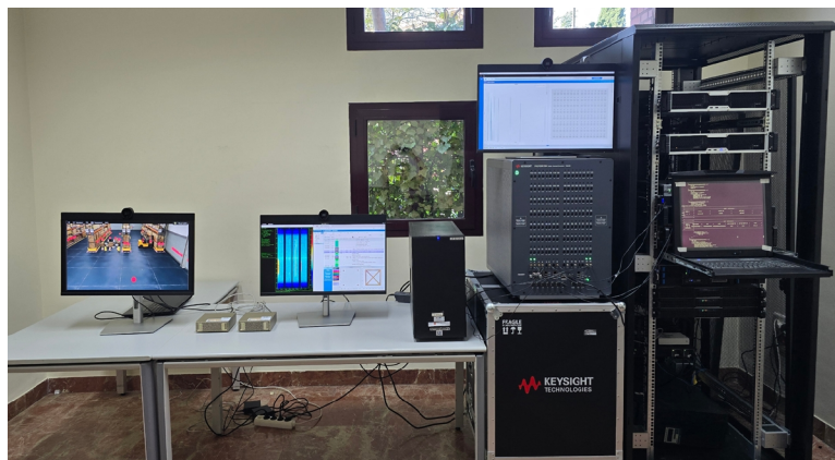
Testbed for software defined radio and channel emulation - Credit: Pablo Picazo, UC3M.
